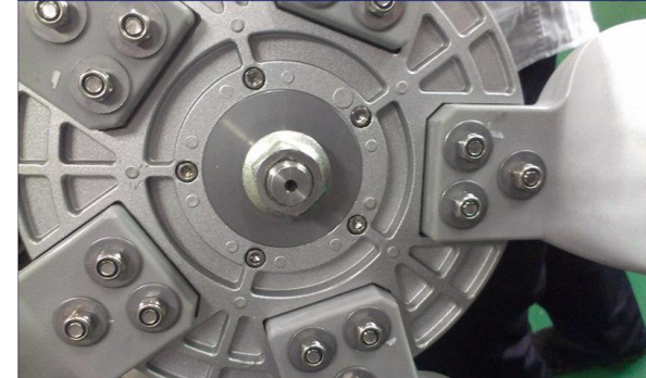
③ Fully tighten the nut to 290N.m
