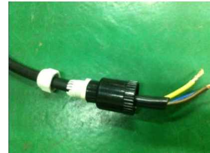
③ Pass the wires through the cover.
