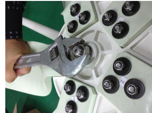
③ Fully tighten the nut to 154N.m
